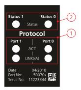
Figure 7: Status LED's on exchangeable cover with Industrial Ethernet
