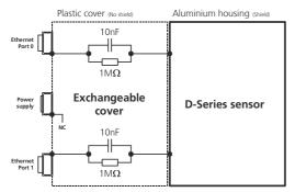
Figure 6: Shielding concept of the D-Series sensor and the exchangeable cover with Industrial Ethernet
