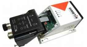
3) Connect the ribbon cable (20 conductors) of the exchangeable cover with Industrial Ethernet to the D-Series device. The connection of the ribbon cable is shown on the left.
