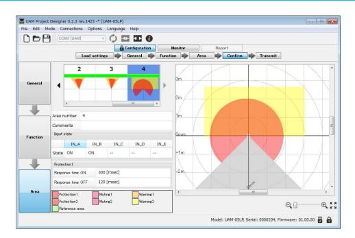
Figure 7-48 Confirm monitor example
