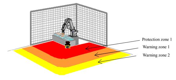
Figure 4-1 Example of access protection
