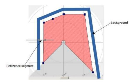
Figure 3-7 Protection zone configured using teaching mode
