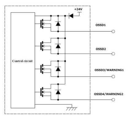
Figure 6-6 OSSD/WARNING Output circuit
