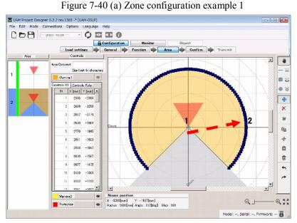
When mouse is dragged from point  $1 \rightarrow$  point 2, a circular shape with origin at point1 is generated. Circular shape cannot be formed if point is dragged beyond the allowed region. Coordinates of each point are also displayed on the coordinate panel. Points are displayed at every 2.5°.
