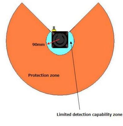
Figure 5-9 Limited detection capability zone
