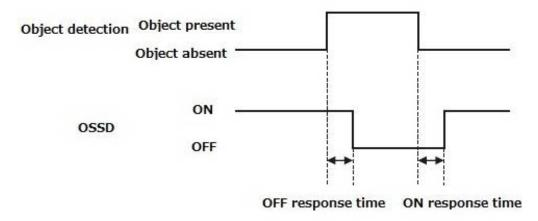
Figure 3-15 Timing chart of automatic restart
