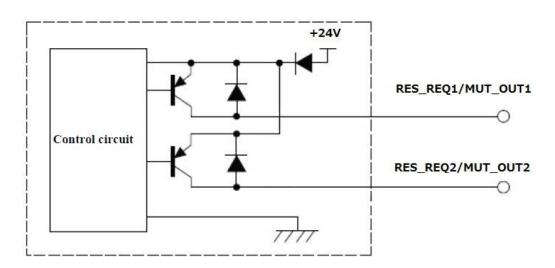
Figure 6-7 Output circuit
