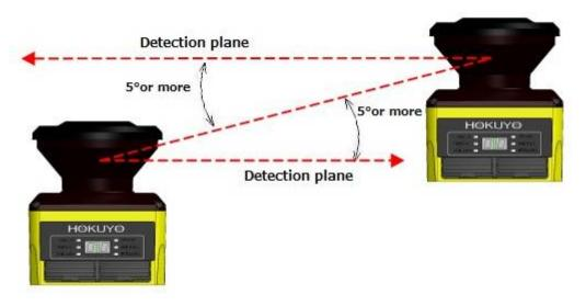
Figure 5-3 Parallel installation
