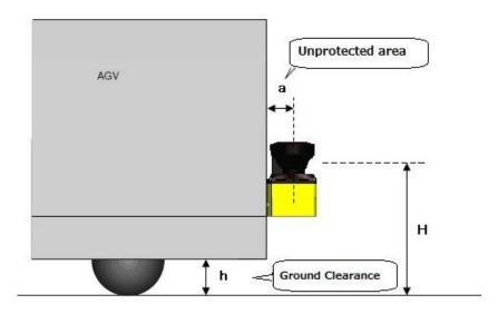
Figure 4-12 Side view of area protection (Mobile)
