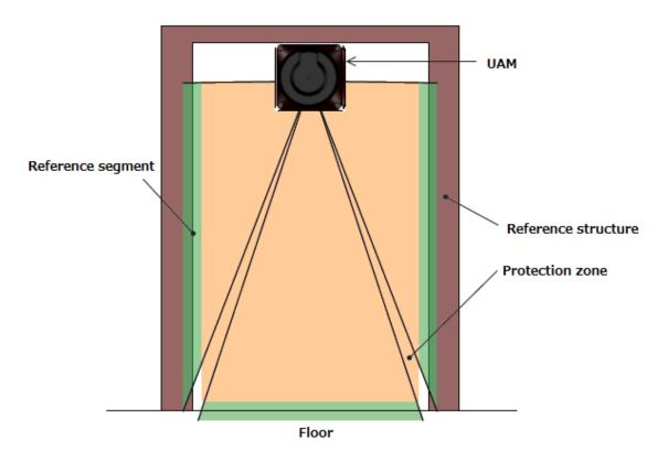
Figure 3-23 (b) Front view of the access detection using reference monitor function
