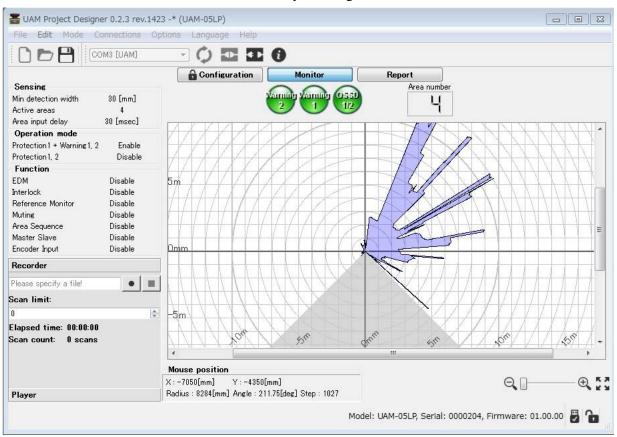
User can monitor the detection state of the UAM by selecting the monitor tab.
