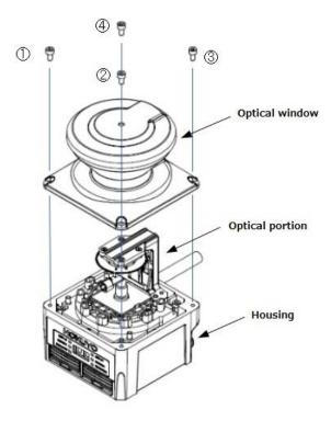
Figure 8-1 Remove the optical window
