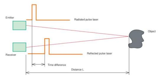
Figure 3-5 TOF operation principle
