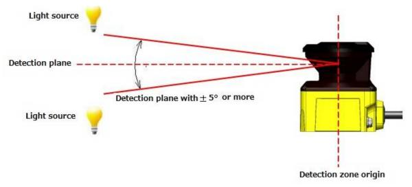
Figure 5-1 Installation to avoid light interference
