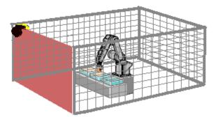
Figure 4-5 Example of access protection (Whole body detection)
