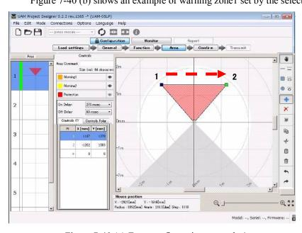
When a straight line is drawn from point  $1 \rightarrow$  point 2, a triangular shape is formed by connecting these two lines with origin. Coordinates of point 1 and point 2 are also displayed.
