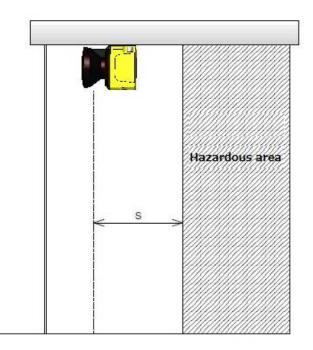
Figure 4-7 Side view of access protection (Whole body detection)
