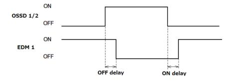
Figure 3-19 EDM timing chart
