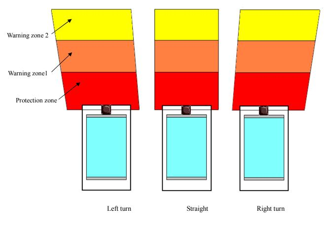
Figure 4-14 one example of AGV scanning area at curve (Top view)
