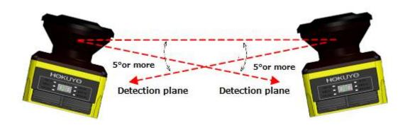
Figure 5-5 Parallel installation
