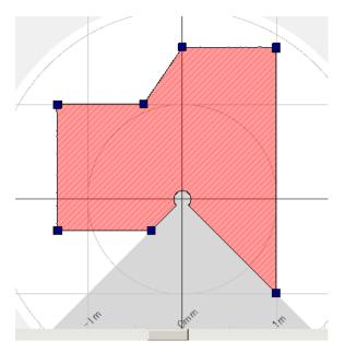
Figure 3-6 Protection zone configured using manual mode
