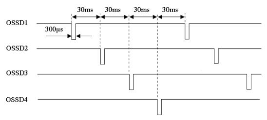
Figure 3-14 Timing chart of the OSSD's self-diagnostic function
