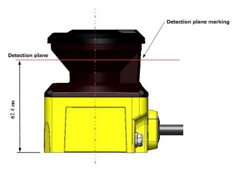
Figure 3-3 Detection plane of UAM-05LP (Side view)
