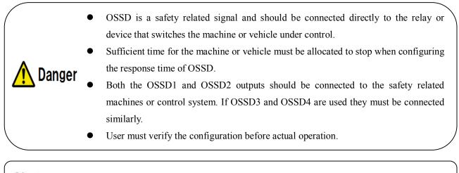
**Note** • When OSSD is at ON state, the signal is 24V and the signal is 0V during OFF state.
