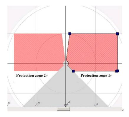
Figure 3-8 Example of Dual protection zone configuration
