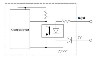
Figure 6-8 Input circuit
