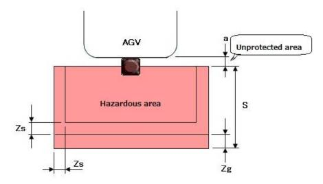
Figure 4-11 Top view of area protection (Mobile)
