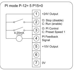
Pressure Control – Variable PI Setpoint with local/remote operation.
