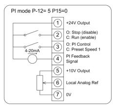
Remote Control (PI) Local Control Control set by pressure level Speed Set by Preset Speed 1 (P-20)
