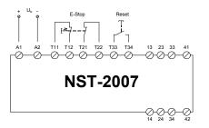
2-channel operation with external contacts, contact monitoring and short circuit protection
