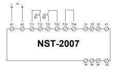
2-channel door monitoring with short circuit protection.
