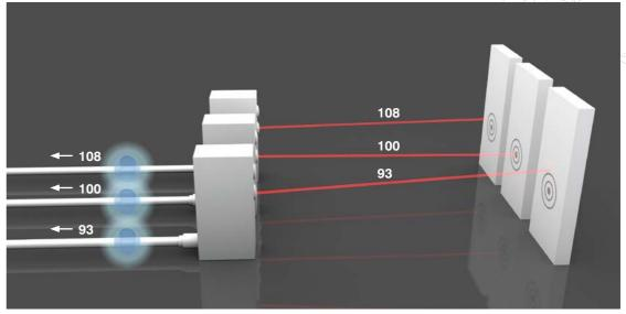
The position of the spot varies in the case of sensors without targeted optics. Acquired data vary as well in the case of non-balanced switching points. Consequently, data communicated from different sensors are not comparable.
