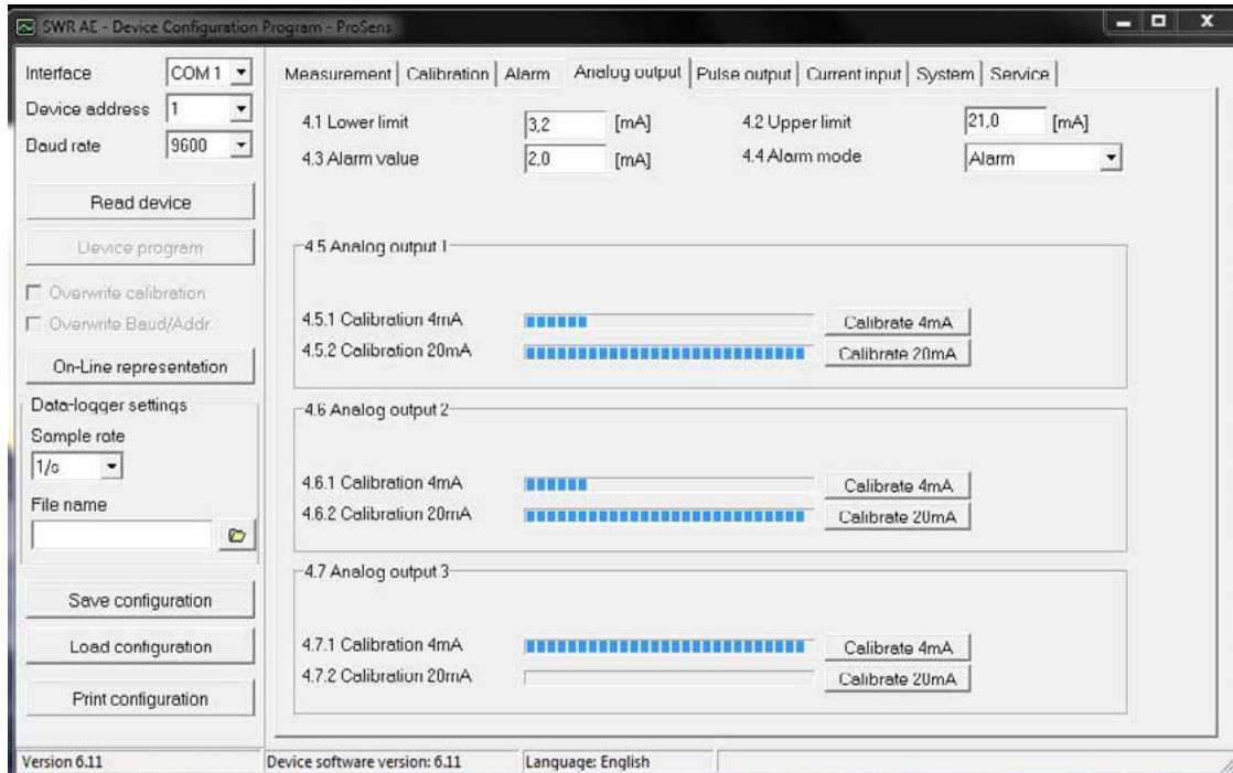
Tab 4: Analogue output Setting and calibrating the analogue output.
