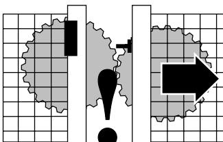
Check the machine is isolated and stopped whenever the interlocked guard door is open.
