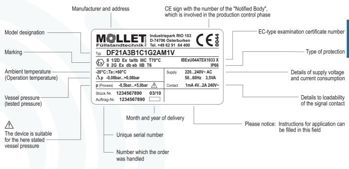
Rotary blade level indicator as electrical device for use on the boundary from zone 0 and zone 20 to zone 1 and zone 21.
