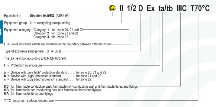
Rotary blade level indicators as electrical devices for use in zone 1.
